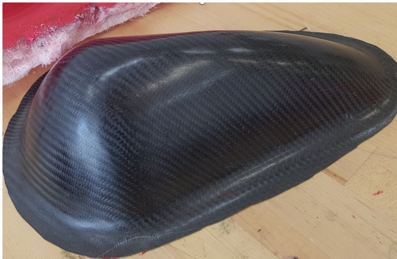
Figure 13: Final composite aeroshell prototype
