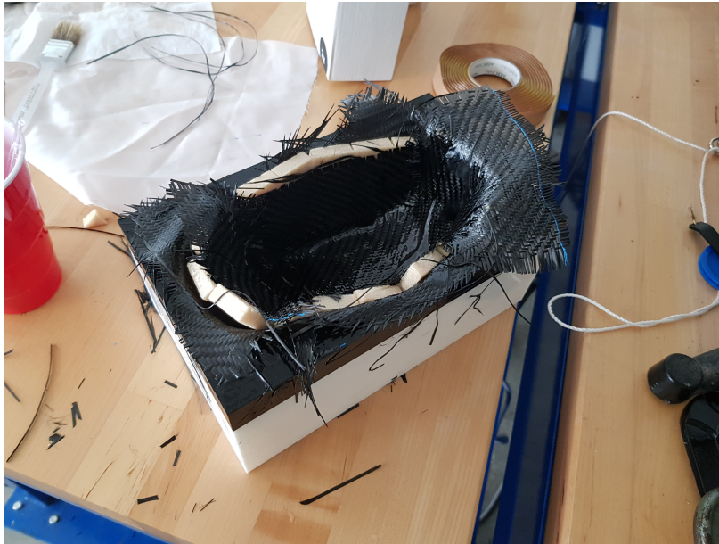
Figure 20: Failed attempt to directly use 3D print as female mold
