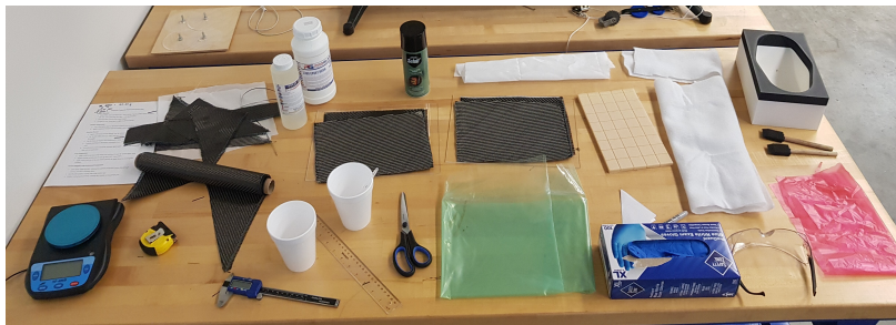
Figure 1: Materials cut and prepped for wet layup process
