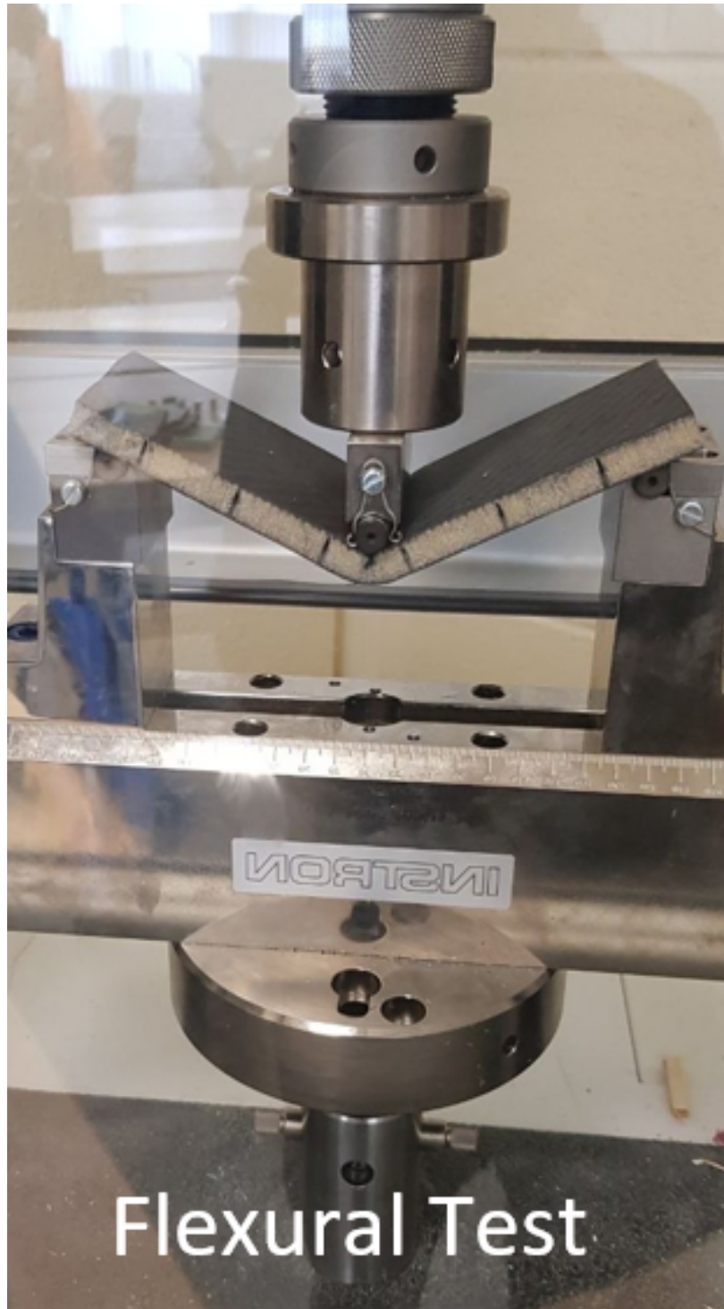
Figure 22: Flexural Test Set up
