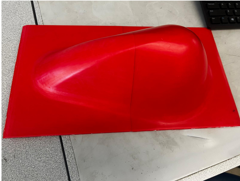
Figure 6: 3D printed pattern prepared for mold making
