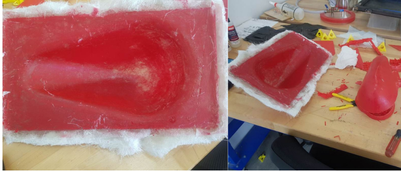
Figure 9: Demolding the female mold from the plug
