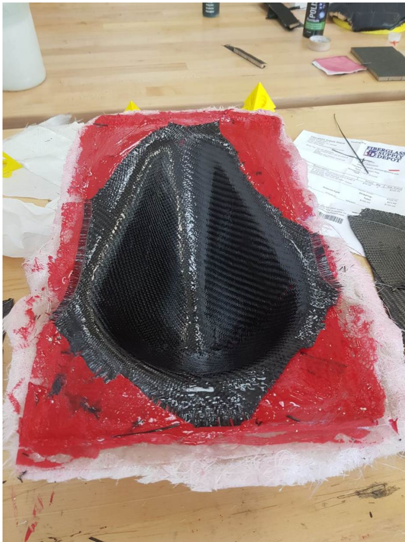
Figure 11: Small Scale Aeroshell Canopy lay up inside the female mold
