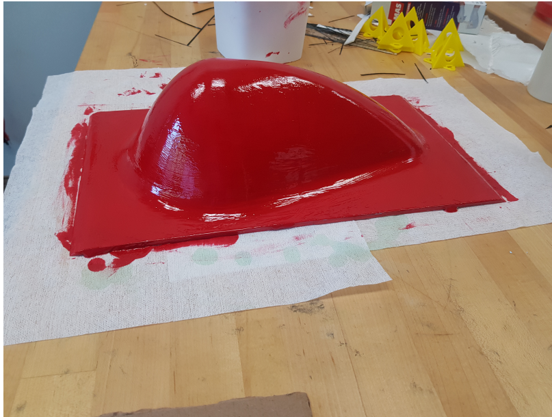
Figure 7: Tooling gelcoat applied to the plug
