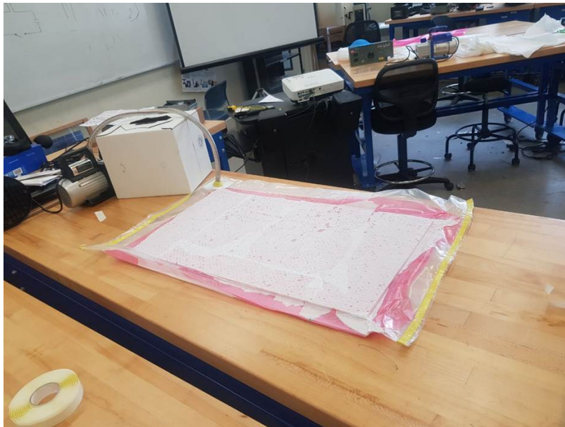
Figure 2: Vacuum bagging setup for composite curing
