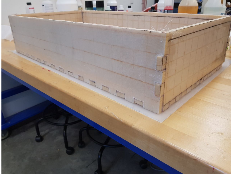
Figure 4: Epoxy bonding of battery box joints
