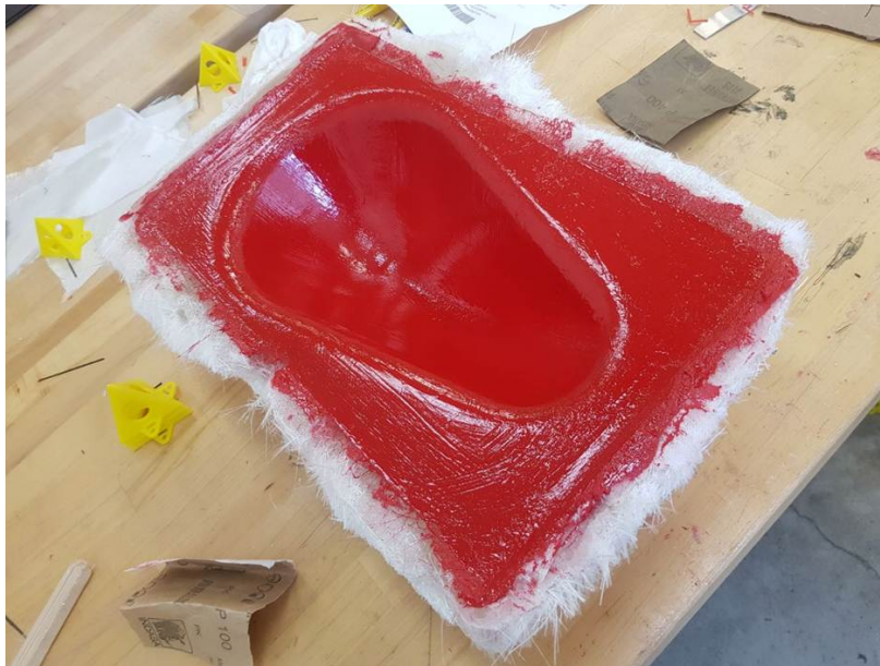
Figure 10: Female mold coated with tooling gelcoat after demolding
