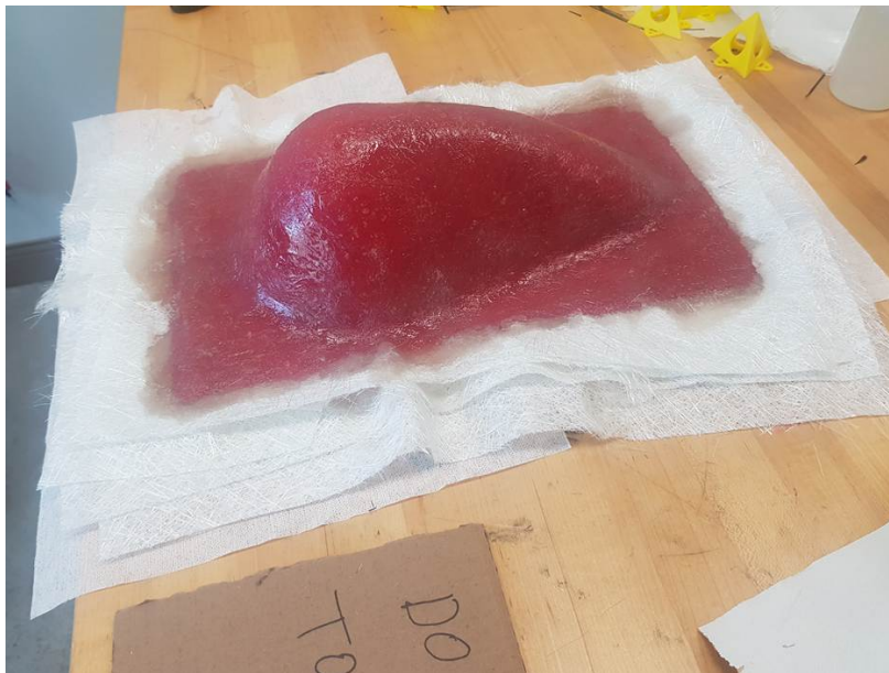
Figure 8: Female mold fabrication using gelcoat and fiberglass
