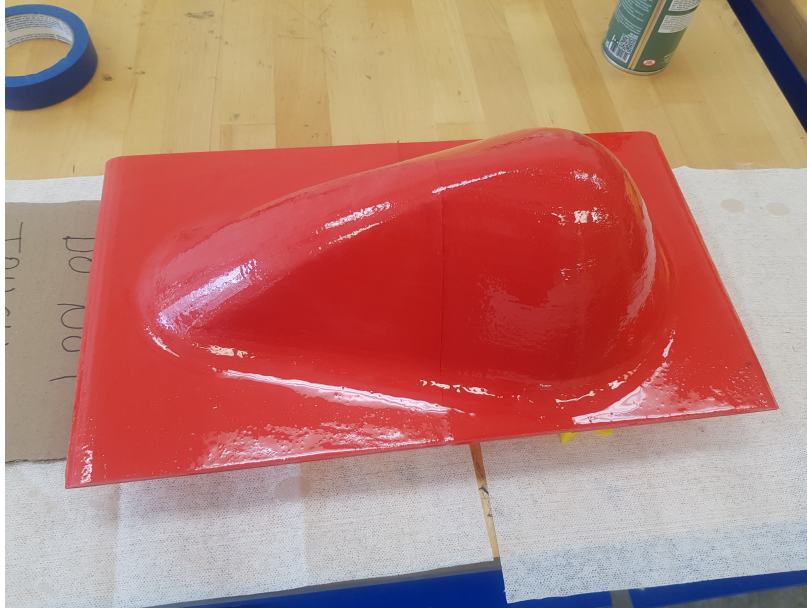
Figure 5: 3D printed pattern coated with epoxy coating
